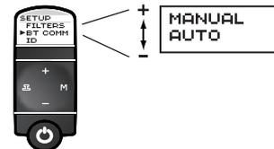
**To obtain model and software version information:** Select the ID option in the SETUP menu. Use the (-) and (+) buttons to scroll through the list of reference numbers. Press “M” to return to the operating mode of the stethoscope.
