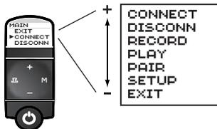
**To enter the Setup Menu:** Use the (-) button to scroll down the list of Special Functions until SETUP is highlighted. Select the SETUP option by pressing and releasing the (M) button. This will display the following menu:
