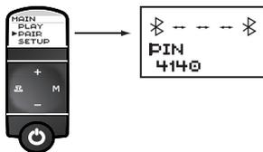
During the pairing process the Model 3200 will make itself discoverable to other Bluetooth equipped devices.
