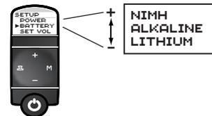
**To specify the preset (default) volume level:** Select the SET VOL option in the SETUP menu. Press and release the (M) button to select the current volume level as default. The factory default is level 3.
