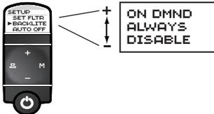
**To select auto off power management:** Select the AUTO OFF option in the SETUP menu. Use the (-) and (+) buttons to scroll through the list of options. Press and release the (M) button to select. The factory default is ENABLE.
