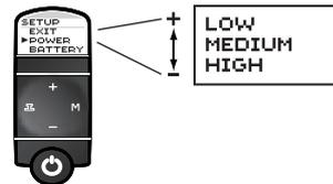
The power settings provide different degrees of power consumption. In general, the longer the stethoscope remains in an active mode, the greater its power consumption. The factory default is the MEDIUM level. (NOTE: The Auto Off power management feature is further described below).
