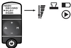
2. **End playback:** Depress and release the (M) button. The stethoscope will stop playing the sound track and will return to its previous operational mode.
