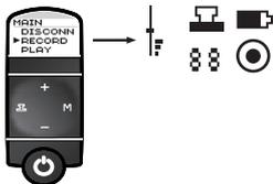
3. **End the recording:** Depress and release the (M) button. The stethoscope will stop recording and the recording icon will disappear from the LCD display. If the time between the beginning and ending of the recording session is greater than 29 seconds, only the last 29 seconds will be saved.
