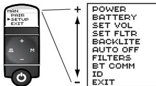
**To select the power setting:** Select the POWER option in the SETUP menu. Use the (-) and (+) buttons to scroll through the list of power settings. Press and release the (M) button to select a setting.
