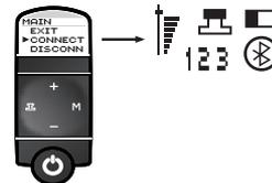
When connected by a Bluetooth link, external Bluetooth-enabled devices may take control of the display and keypad of the Model 3200 stethoscope. The external device may also transfer audio playback or other information through the Model 3200 headset. When the external device transfers audio playback back to the stethoscope, the sounds will be preceded by a beep.
