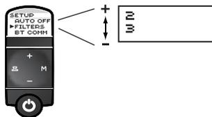
**To specify Bluetooth mode:** Select the BT COMM option in the SETUP menu. Use the (-) and (+) buttons to scroll through the list of options. The MANUAL option means that the Bluetooth link can be used for data transfers but requires user activation. The AUTO option means that the Bluetooth link is continuously powered and ready to connect to an external device which it has been previously paired. Press and release the (M) button to select an option. The factory default is MANUAL.
