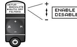
Two different settings work together to influence the length of time the Model 3200 is on full power: The AUTO OFF setting (ENABLE vs. DISABLE) and the POWER setting (HIGH, MEDIUM, and LOW - HIGH setting uses more battery power, LOW setting uses less battery power). To increase battery life, ENABLE the AUTO OFF feature and select the LOW power setting.
